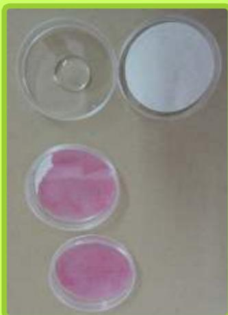
1. Add 1 ml of sample (or appropriate dilution) in the center of the plate.
